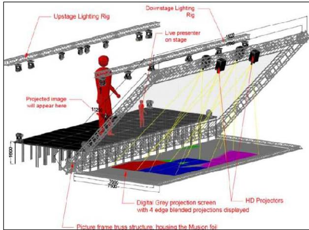
Figure 4 - Drawing of a typical Musion Eyeliner stage production
